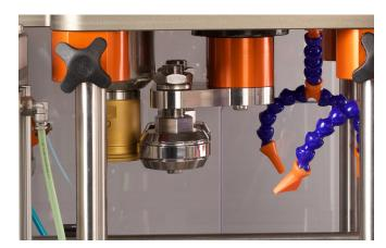
Seaming on the IMP2 is completed effortlessly and accurately due to our revolutionary new electronic seamer. The proven system provides industry standard double seams that can be compared to any high end multi head machines. Microcan have developed seamer tooling with a proven extensive double lifespan. If adjustments are required, they can be carried out simply on screen to maintain high tolerances.
